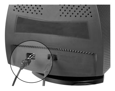
**5** Plug the other end of the power cord into a correctly grounded electrical outlet.
